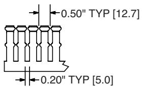
Multiple slot restrictors present with 62mm and greater duct wall height.
