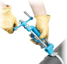
2) Insert tail of strapping into tool nose section. Rotate handle to tension.
