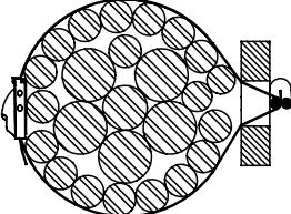
6) Install cable tie around bundle and fasten.
