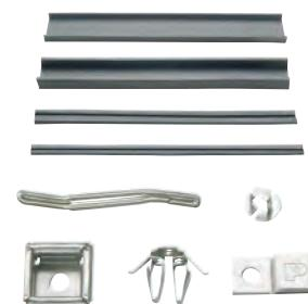
Pan-Steel® System Accessories are used with Pan-Steel® Stainless Steel Cable Ties to speed and simplify the mounting of wires, cables, and tubing. Installation methods include screw mounts and push mounts. See pages B3.22 – B3.25.
