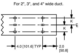
**Panduct® Type HN Wiring Duct Dimensions**
