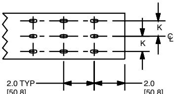
Note: For type FS wiring duct, no mounting holes is the standard condition; if mounting holes are required, delete NM from the part number.
