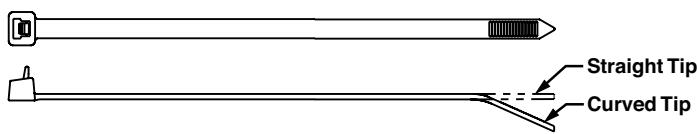
To release, grasp the head of the cable tie, deflect release tab, and pull the cable tie away from the bundle.
