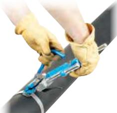
3) After tensioning raise tool 90° – 120° over buckle and pull down on cutter lever, cutting strap.
