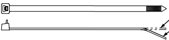
To release, grasp the head of the cable tie, deflect release tab, and pull the cable tie away from the bundle.
