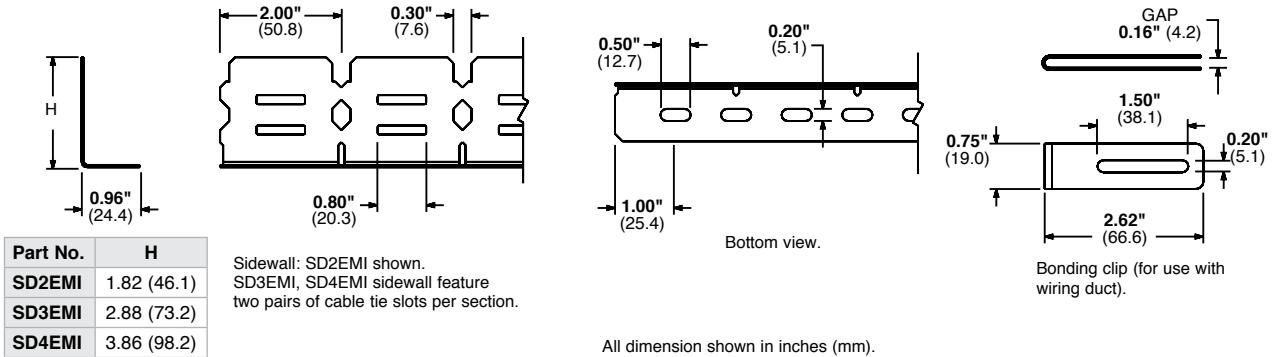
**Panduct® PanelMax™ Corner Wiring Duct Dimensions**
