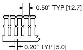
Multiple slot restrictors present with 2" and greater duct wall height.
