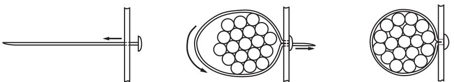
1) Insert tip of cable tie through the pre-drilled hole in the panel.
