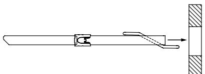
2) Insert cable tie and mount through panel/framework hole.
