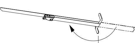
1) Insert cable tie through mount slot and fold cable tie.
