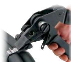
1) Place strap around the material, insert tail of strap through buckle. Pull strapping tight and bend up to hold in place. Insert tail of strapping into tool nose section. Squeeze handle to tension.
