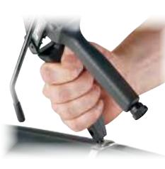
4) Using the closure lever on the handle of the tool, bend retaining tab down and over cut end.
