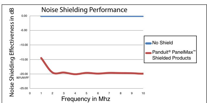
Relative noise reduction in decibels over frequency range of Panduit® PanelMax™ Shielded Wiring Duct and Noise Shield
