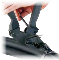
2) Once proper tension is reached, maintain tension and raise tool 90° – 120° over buckle and pull down on cutter lever, cutting strap.
