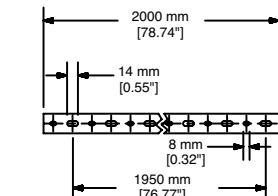
For 75mm and 100mm width duct.
