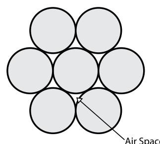
In our wirefill formula an adjustment is made to the channel internal area to account for "unusable" air space that will be present between cables when placed in the channel. Our formula assumes a uniform close packed or high-density cable arrangement (see diagram) (Note 1).
