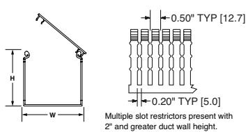
Multiple slot restrictors present with 2" and greater duct wall height.
